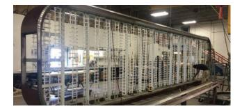
SignBOX II is recommended for installation 300 mm (12") on center for depths of 125 - 150 mm (5 - 6") from face, as this yields the same brightness as a fluorescent lit cabinet; however, in deeper cabinets at 200 - 230 mm (8 - 9") from face, the spacing may be spread further to 350 - 400 mm (14 - 16") on center, saving product, time, and money.
