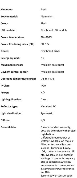
System power consumption (LED module & driver) depends on components used
